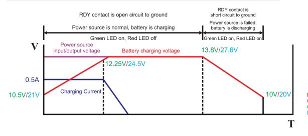
Battery Charging Voltage Curve (Red Line): Green: 12V Light Blue: 24V
